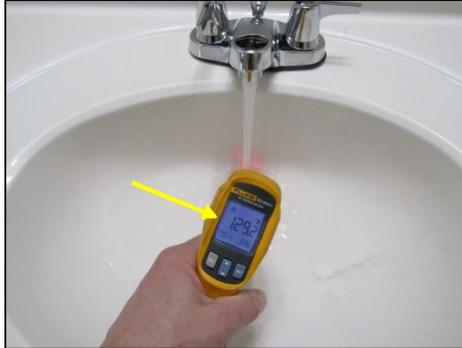
High water temperature noted. Recommend between 113 F and 125° F for the safety of children. Water temperature can be adjusted at the water heater.
