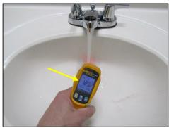
High water temperature noted. Recommend between 113 F and 125° F for the safety of children. Water temperature can be adjusted at the water heater.
