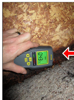
9.1 HOUSE FLOOR SLAB (Picture 2) High moisture
