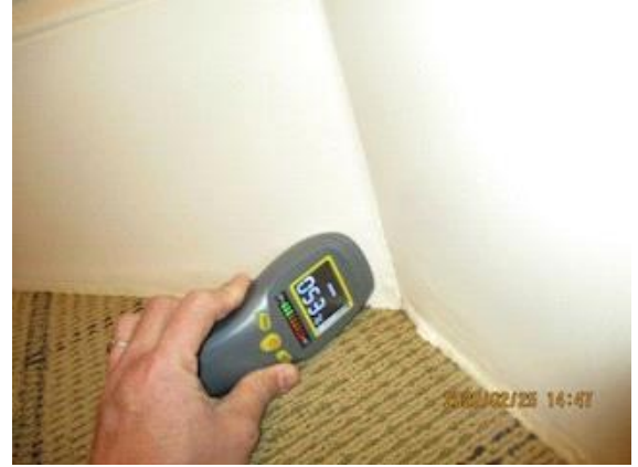
Basement grand room : Elevated moisture detected at the baseboard
