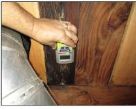
Active leak, moisture meter reads 100%
