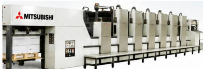
One of the 6-color commercial presses used by Allan Kullen's printing company.
